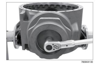
④ Heat the tapered roller bearing and insert it into the input pinion until contact is obtained.
