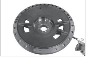
6 Lift differential out of the axle drive housing with the lifting device.
