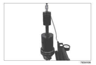
Is Loosen the threaded connection and remove the releasing oil tube.
