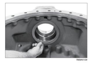
③ Undercool the internal bearing outer ring and bring it into contact position in the housing hole by using the assembly fixture.
