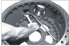
If necessary pull the internal bearing outer ring out of the axle drive housing and remove the shim behind.
