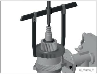
Pull off bearing inner ring with 5873.012.019 [Rapid grip] and 5873.002.000 [Basic tool].
