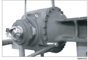
② Fix axle drive housing to the assembly truck.
