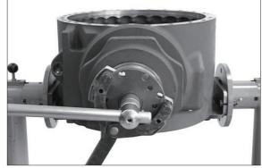
① Pull input flange from the input pinion and use a lever to lift the shaft seal ring behind out of the axle drive housing.
