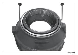
② Use a lever to remove the slide ring seal from the output shaft.
