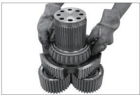
(6) Wet front face (contact face bearing inner ring, arrow 1) and profile (teeth, arrow 1) in the output shaft with anticorrosive agent.
