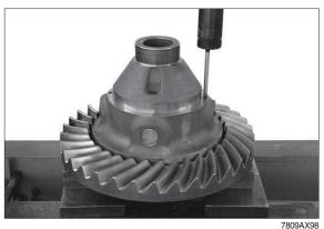
10 Pull spider shafts (4EA) and remove the releasing spider gears with the thrust washers from the differential housing.
